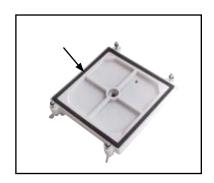
**Step 7**Fit lid checking for correct positioning. Evenly tighten in the sequence shown.
